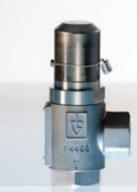
418 Overflow valve of high-quality stainless steel design. Another highlight in the product program of Gerhard Götze KG: This bypass overflow valve of stainless steel features a replacement cartridge. The valve incorporated in the piping system therefore remains untouched during any revision work - just the cartridge is replaced. Gerhard Götze KG has simply trans ferred this facilitation, long used in heating installations, to industrial
